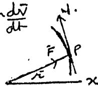
$$\therefore \frac{d}{dt}(\bar{r} \times \bar{v}) = \frac{d\bar{r}}{dt} \times \bar{v} + \bar{r} \times \frac{d\bar{v}}{dt}$$
