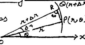
The area swept by the radius of a particle in unit time is called Areal Speed
