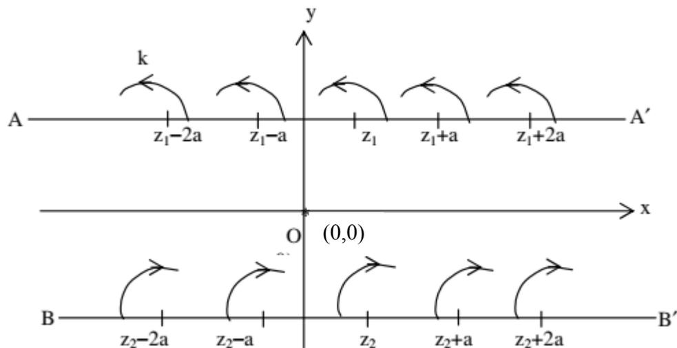
Let one vortex on infinite row  $AA'$  be at  $z = z_1$  and one vortex on infinite row  $BB'$  be at  $z = z_2$ , so that the system consists of vortices  $K$  at  $z = z_1 \pm na$  and vortices ' $-K$ ' at  $z = z_2 \pm na$ ,  $n = 1, 2, \dots$
